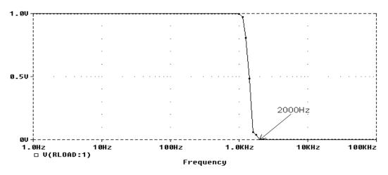
• Examine circuit's behavior for each of 101 frequency values chosen over five decades of frequency (from 1 Hz to 100,000 Hz) with each decade divided into 20 parts (using a logarithmic scale). The fitness measure
