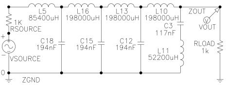
• Replace each of the three 198,000  $\mu$ H inductors in the figure with a series composition of two 99,000  $\mu$ H inductors.
