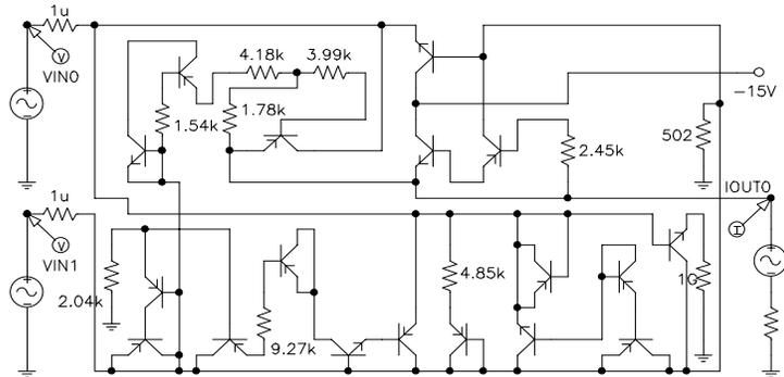
Figure 1. Best-of-run voltage-current-conversion circuit from generation 109
