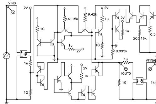
Figure 3. Best-of-run cubic signal generation circuit from generation 182
