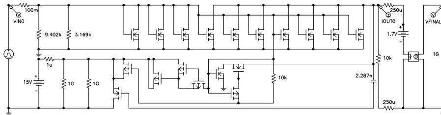
Figure 5. Best-of-run high current load circuit from generation 114
