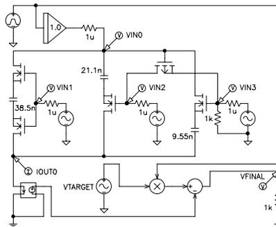
Figure 4. Smallest compliant register-controlled capacitor circuit from generation 98
