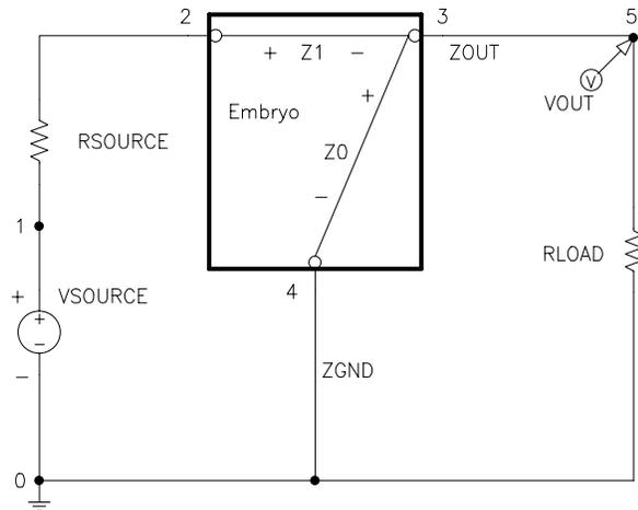
Figure 1 One-input, one-output initial circuit.
