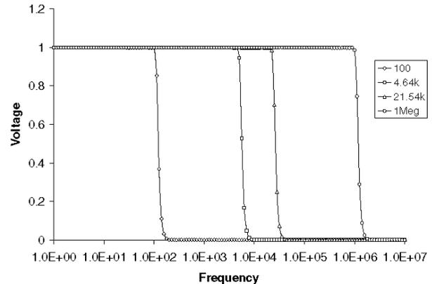
**Figure 4** Frequency domain behavior of genetically evolved parameterized filter for four out-of-sample values of frequency  $f$ .
