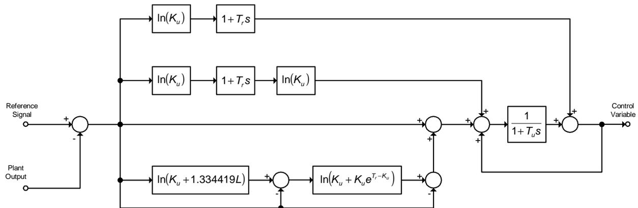
Figure 4 Block diagram of best-of-run controller from generation 217.
