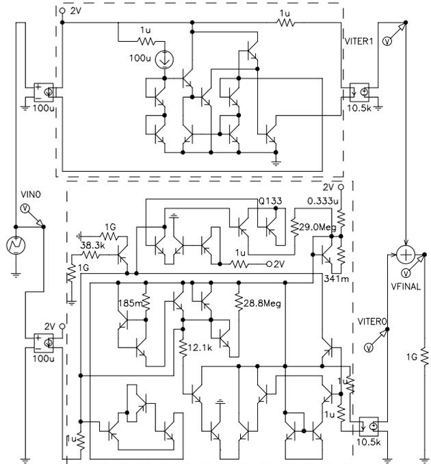
Figure 9: Refined Low-Voltage Cubic Signal Generator Circuit
